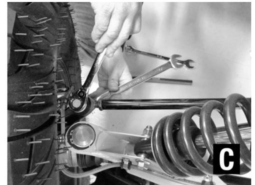
**Step 5:** Remove tie rod end from factory tie rod by spinning to loosen/un-thread. Set tie rod end aside it will be re-used. (Figure D)
