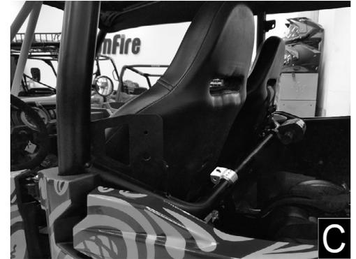
**Step 5:** Obtain Eyelet bolt [P3], washer [P5], and locknut [P6]. Place Eyelet Bolt [P3] through hole in bracket and then install with hardware (Figure D).
