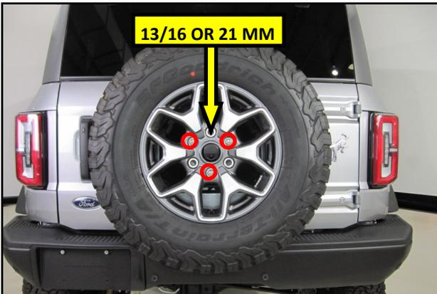
**1.** With the vehicle parked on level ground, open the tailgate approx. 5 to 10 degrees and remove the spare tire. Note the movement in the tailgate due to the spare tire removal. The noted movement due to tire weight should be accounted for during final alignment.
