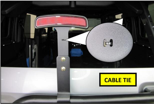
47. Secure the wire harness to the Upper Brake Light Bracket using the supplied Cable Tie. Trim the excess length.
