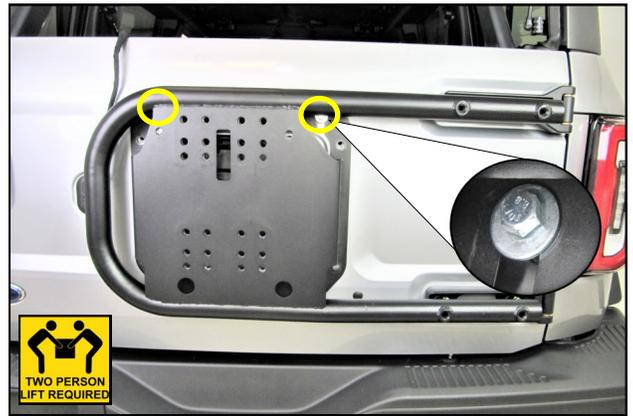
**30.** With help from an assistant, carefully lower the Tire Carrier Hoop onto the hardware from step 28 and into the RTR Hinges.
