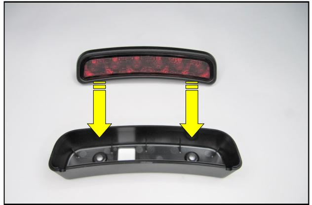
42. Place the OEM brake light into the RTR Brake Light Housing.
