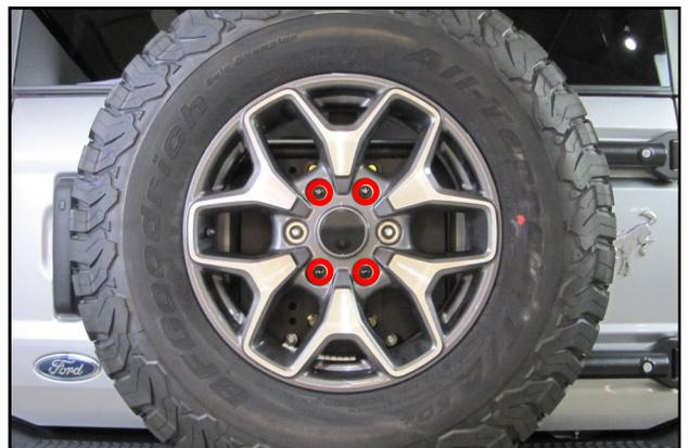
52. Using four of the supplied Spline Drive Lug Nuts and Socket, snug the spare tire down onto the RTR Tire Carriers Hub.
