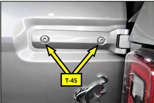
19. Using a T-45 TORX® driver, remove the two upper exterior hinge bolts and set the hinge aside. The OEM hinge and hardware will not be reused in this installation.
