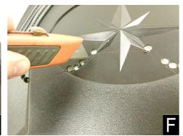
Step 7: Once the center of the cutout is removed, you may need to do some final trimming to allow the bezel to fit with minimum resistance.
