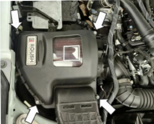
6. Start the vehicle and check for any leaks around air box lid. Make sure that the seal has not been distorted during installation.
