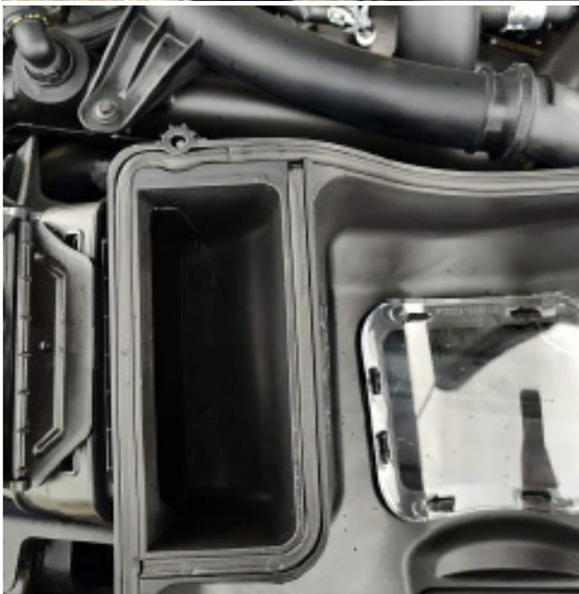
4. Snap the new air box lid (PT00041966) onto the rubber snorkel inlet.
