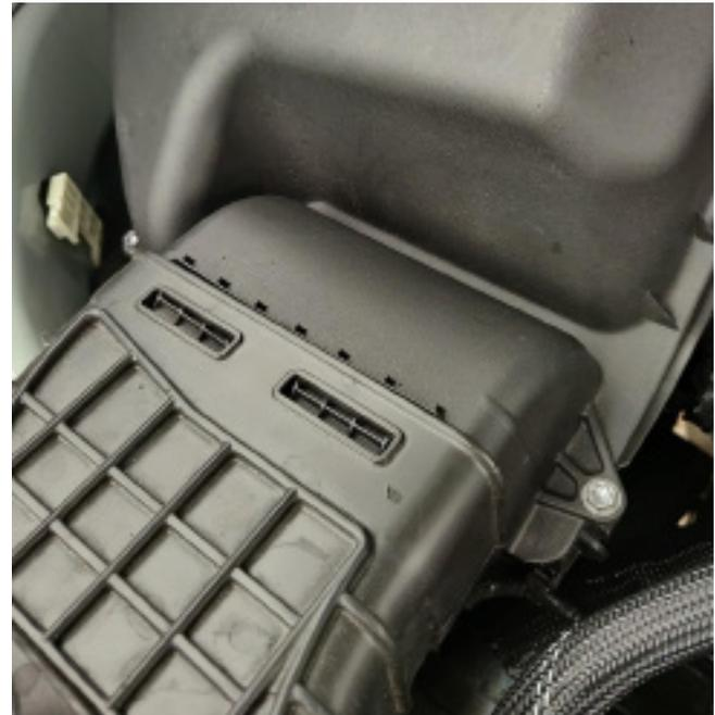
5. Install the lid onto the lower air box tray using the four (4) screws removed previously. Torque to 3Nm.
