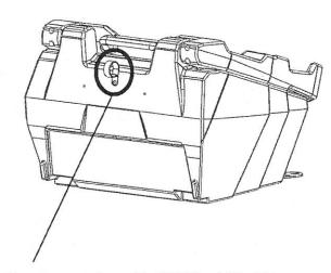
Clamp fastener to be used for RZR 570 and 800 vehicles.
