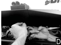
Step 6: Place additional weather stripping where roof contacts roll cage. Install two P-clamps[P5] to roll cage at front visor and middle section seam and align to outter holes. Attach with button head screws[P6] and washer[P8] from top side, then secure through P-clamp holes with nylon locknut[P9] from underneath. (Figure E)
