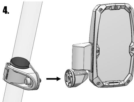
Using an 8mm Allen wrench, screw the bolt into the mirror but do not tighten yet.
