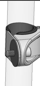
Close clamp around roll cage tube, put the bolt through the hole, and place large rubber washer over the end of the bolt.
