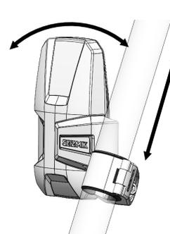
Rotate mirror on clamp so that it is level. When you are satisfied with the location and angle, tighten bolt.
