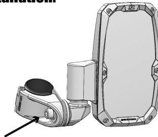
Temporarily remove this socket head bolt using an 8mm Allen Wrench
