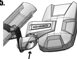
To tighten the folding feature of the mirror, tighten tension adjustment nut on the bottom of the mirror arm.
