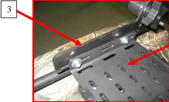
FYI: The Gear Lock and Load Plate (Sold Separately) is made to accept the Metal Mounting Plate. Simply slide the Mounting Plate into the slots of the Gear Lock and Load until you hear it snap. The snap is made by the square hole in the Metal Mounting Plate engaging the tab on the Gear Lock and Load. To remove, press the tab on Gear Lock and Load and slide out the entire Gun Boot Bracket.
