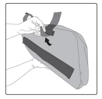
1a) If using Polaris part number 2879509 or RZR4 #2879942 optional lower doors installed pass the middle top strap on bag through the webbing loop on backside first. Then hold bag up to the bottom of the lower frame of the factory door. Pass the 2 upper straps around the door frame and connect the self-fastening straps.
