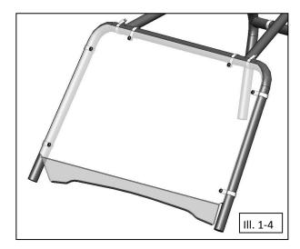
4. Repeat step 3 for remaining 5 Clamps and torque to specifications.
