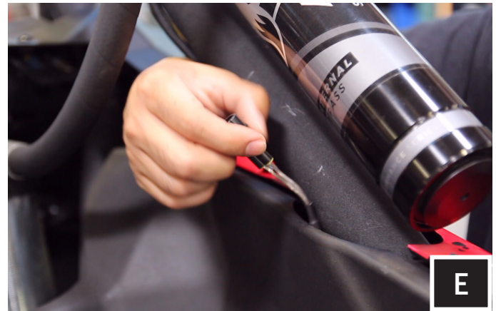
E. Route the rear speaker harness (B-H2936) along the factory wires in the engine compartment and pull up through the small space between the bed panel and cage tubing on both passenger and driver sides.
