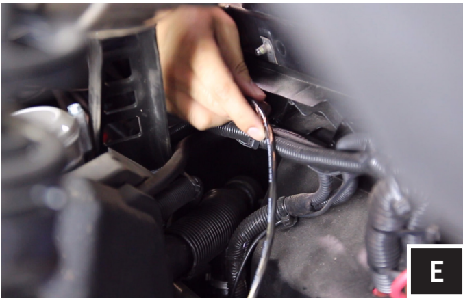
E. Route the rear speaker harness (B-H2936) along the factory wires in the engine compartment and pull up through the small space between the bed panel and cage tubing on both passenger and driver sides.
