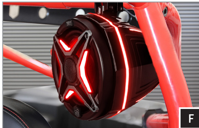
F. Install the speakers to the cage mount and route the speaker wire away from any moving parts and any sharp metal, then connect to the radio or amplifier.
