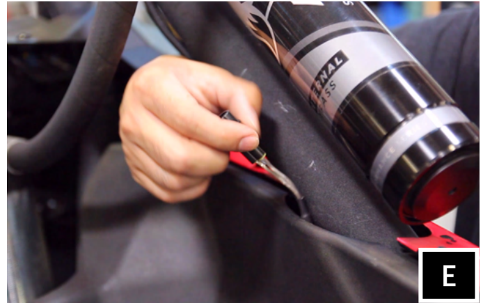
E. Route the RGB LED rear speaker harness (B-H2936) along the factory wires in the engine compartment and pull up through the small space between the bed panel and cage tubing on both passenger and driver sides.
