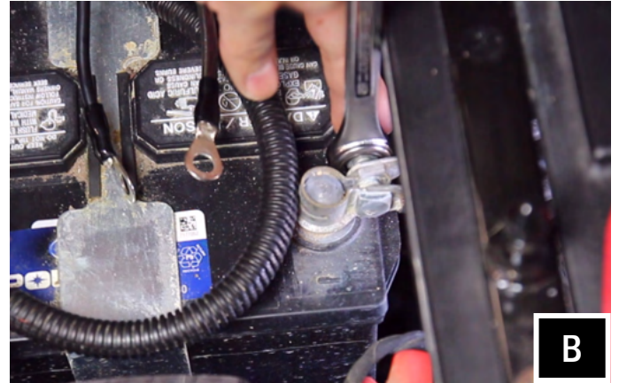
B. Disconnect the negative battery cable from the battery.
