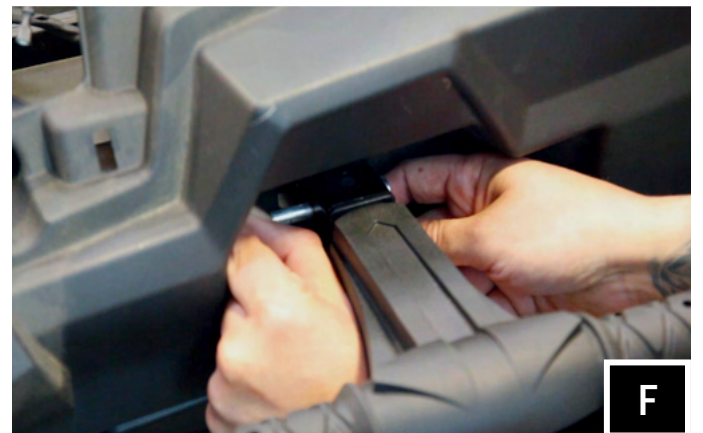
F. Un-pin and pull to remove the passenger side safety handle.
