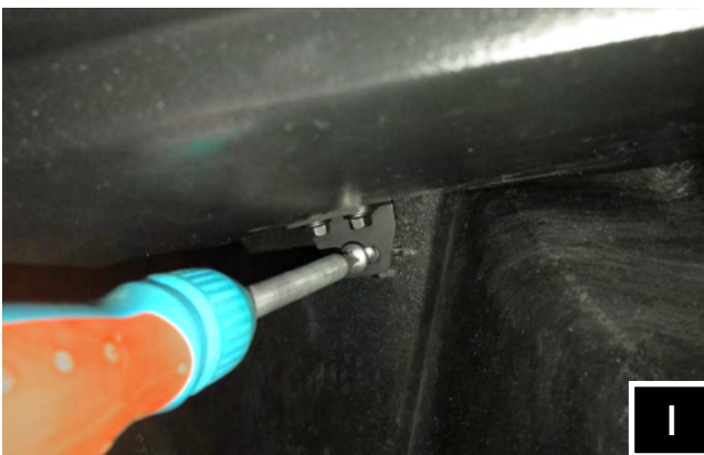
I. Fasten the provided #14 screw to secure the enclosure lower mounting bracket. (RZ4 ONLY)
