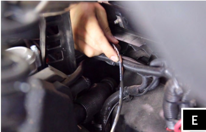
E. Route the RGB LED rear speaker harness (B-H2936) along the factory wires in the engine compartment and pull up through the small space between the bed panel and cage tubing on both passenger and driver sides.
