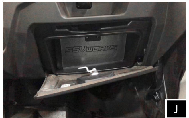
J. Attach the factory glovebox door.
