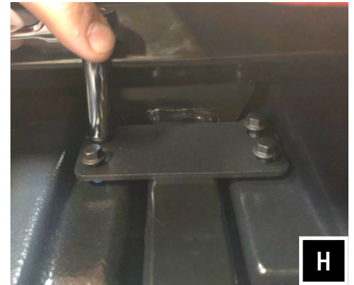
H. Place Bracket "A" into place towards the firewall, and fasten it into place with the (4) 8mm socket head screws and washers provided with the kit.
