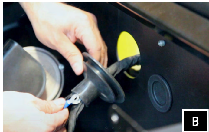
B. Pull the B-H2367 (JVC to SSV harness adapter) POWER and GROUND wires through the rubber grommet and feed through the hole in the firewall to the power strip located on the opposite side of the firewall.
