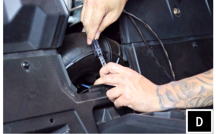
D. Take the B-H2936 RGB LED rear speaker harness and plug into the B-H1913 & B-H1912 rear extension harness.
