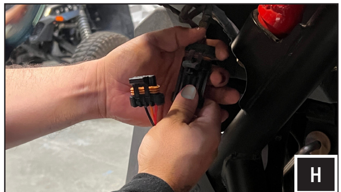
H. Unplug the factory tail light connector and plug it to the "PASS INPUT" connector of the X3 Rear Turn Signal Harness (B-H3205) that was ran to the back of the vehicle on step E.
