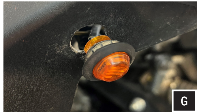
G. Insert the LED turn signal lamp into the hole and push in to lock in place. Repeat steps F and G for the other side.
