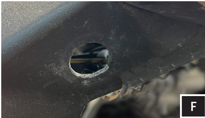
F. Drill a 3/4" hole in the front of the vehicle for the front turn signal LED lamp. Refer to the viewing angle diagram on page 6 for proper turn signal LED lamp placement.
