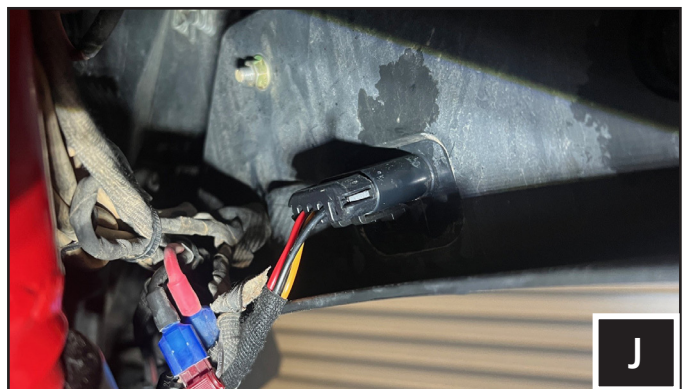
J. Run the "DRIVER OUTPUT" cable to the driver side tail light. Unplug the factory tail light connector and plug in the "DRIVER OUTPUT" connector of the X3 Rear Turn Signal Harness (B-H3205).
