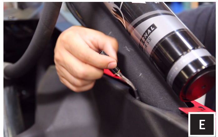
E. Route the rear speaker harness (B-H2195) along the factory wires in the engine compartment and pull up through the small space between the bed panel and cage tubing on both passenger and driver sides.
