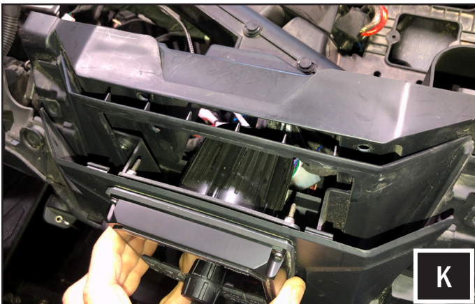
M. Place the assembled RZ5-DMR1 into the dash cavity. It is necessary to angle in one side at a time so that the bracket clears the cavity allowing the dash kit to rest flush. Now complete this step by fully tightening the screws left loose in Step D.
