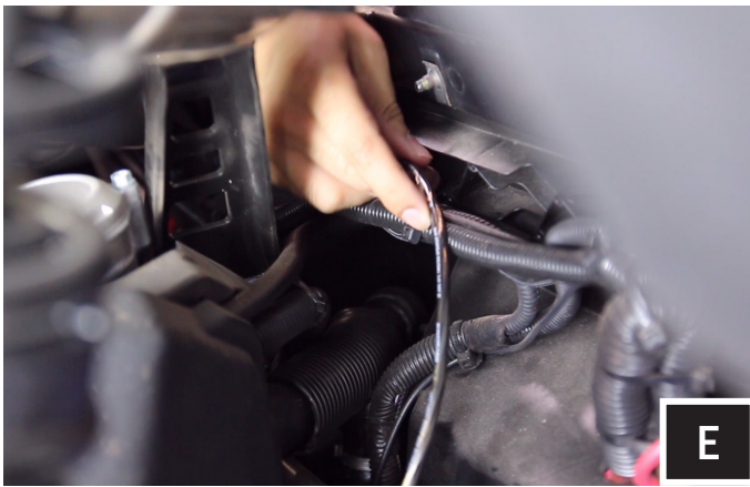
E. Route the rear speaker harness (B-H2195) along the factory wires in the engine compartment and pull up through the small space between the bed panel and cage tubing on both passenger and driver sides.
