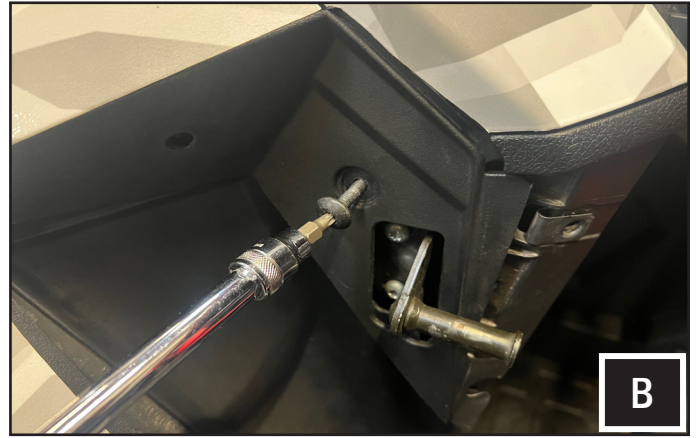
B. Remove the screw holding the door latch panel.
