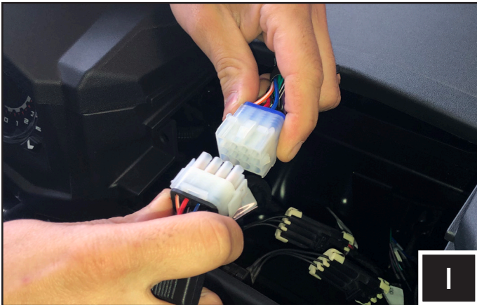
I. Connect the MR1 power harness to the radio harness. Plug the provided universal fm antenna cable if the vehicle does not have an antenna.
