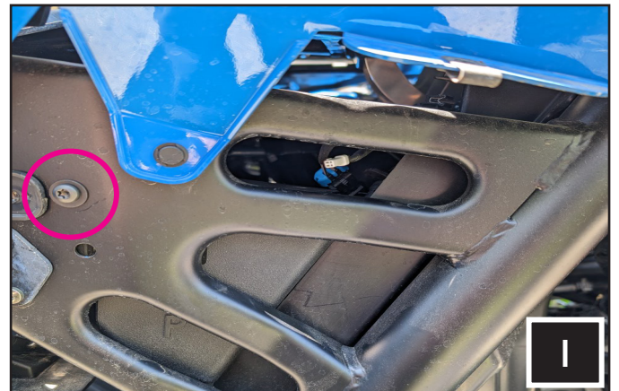
I. Secure the D (driver) and P (passenger) pod brackets to the vehicle frame using (2) M6x16 screws [B-HP3503] circled above.
