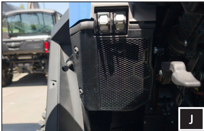
J. Reinstall the factory driver and passenger side speaker grill using the factory screws.
