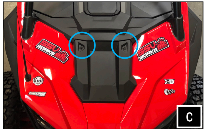
C. Remove the (2) T40 torx screws and set the hood panel aside.
