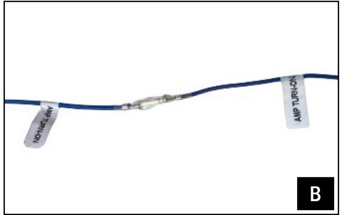
B. Plug the blue Amp Turn on wire of the Anti-Pop circuit to the Kicker amplifier amp turn-on wire.
