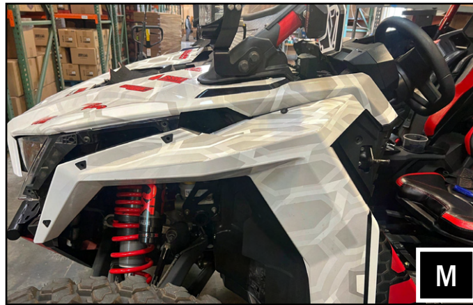
M. Reinstall the front fenders.
