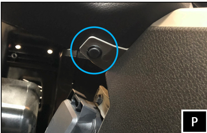
P. Remove the (2) push pins that are found on the bottom of the dash towards the center console.
