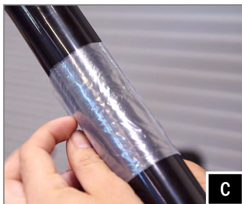
C. Place both ring mounting clamps on the cage using the plastic bag to prevent scratching, place the cage mount pod in its final mounting location and secure to the clamps using the two (2) M6 allen socket head bolts and washers with a 5mm allen key.
