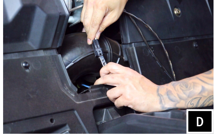
D. Take the B-H2195 rear speaker harness and plug into the B-H1913 & B-H1912 rear extension harness.
