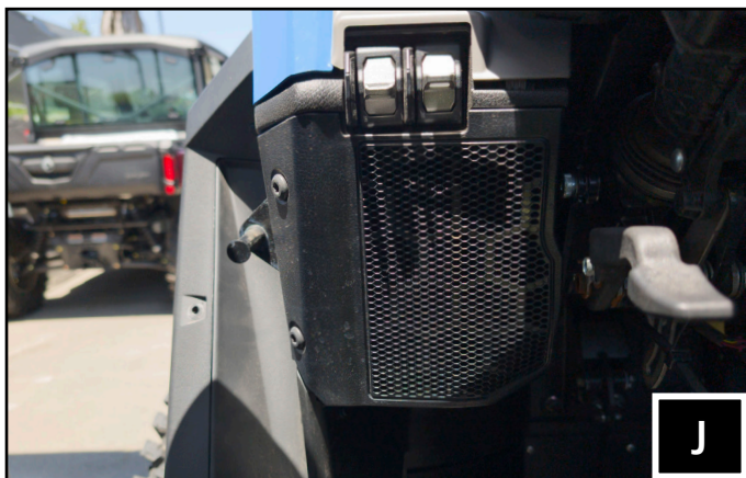
J. Reinstall the factory driver and passenger side speaker grill using the factory screws.
