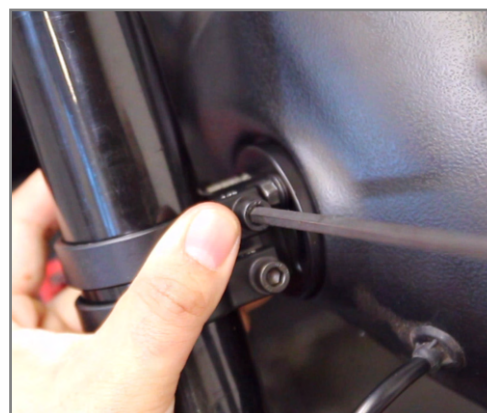
C. Place both ring mounting clamps on the cage using the plastic bag to prevent scratching, place the cage mount pod in its final mounting location and secure to the clamps using the two (2) M6 allen socket head bolts and washers with a 5mm allen key.
