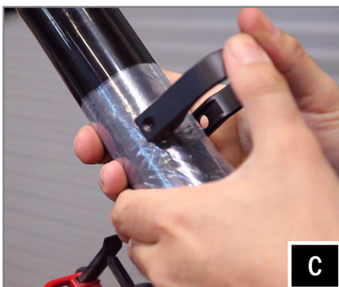
C. Place both ring mounting clamps on the cage using the plastic bag to prevent scratching, place the cage mount pod in its final mounting location and secure to the clamps using the two (2) M6 allen socket head bolts and washers with a 5mm allen key.
