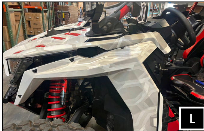
L. Reinstall the front fenders.
