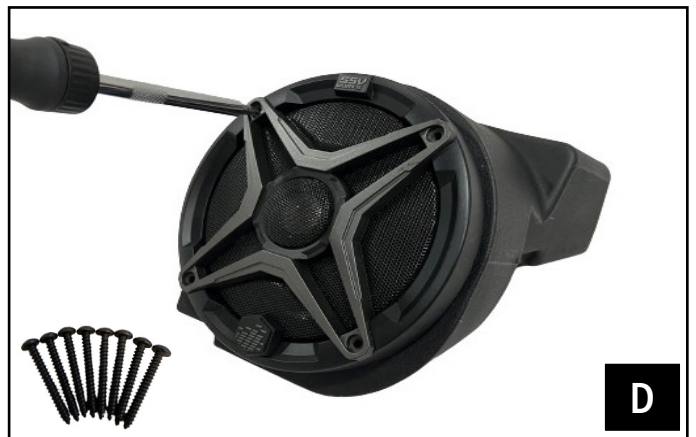
D. Attach the self adhesive speaker gasket and mount the speakers to the dash pods using (8) #7x1.25" screws [B-HP#7-8].
