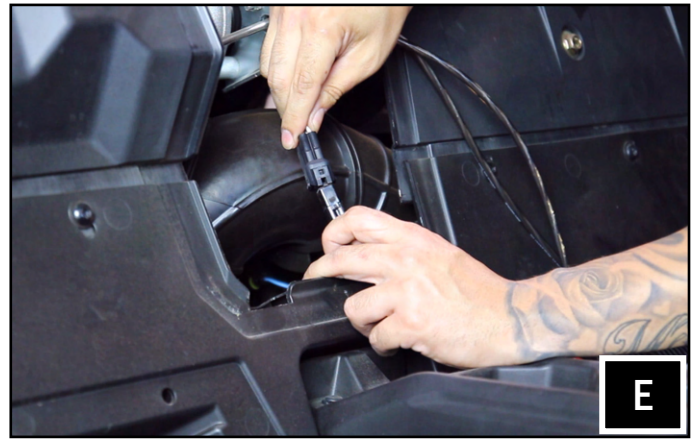
E. Take the B-H2195 rear speaker harness and plug into the B-H1913 (add B-H1912 for 4 door models) rear extension harness. Plug the B-H2936 RGB "Y" harness to B-H2933 (add B-H2934 for 4 door models) RGB extension harness.
