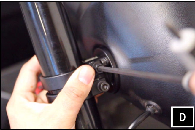
D. Place the cage mount pod in its final mounting location and secure to the clamps using the two (2) M6 allen socket head bolts and washers with a 5mm allen key.
