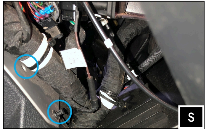
S. Remove the (2) push pins on the passenger side front of the center console.
