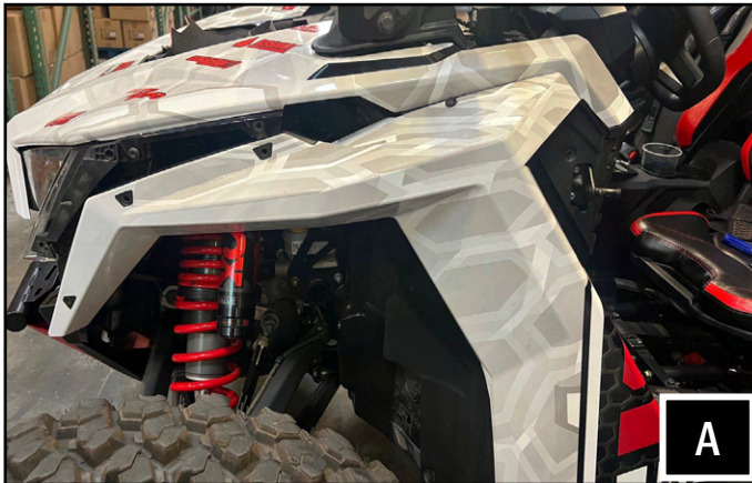
A. Start by removing the front fenders.
