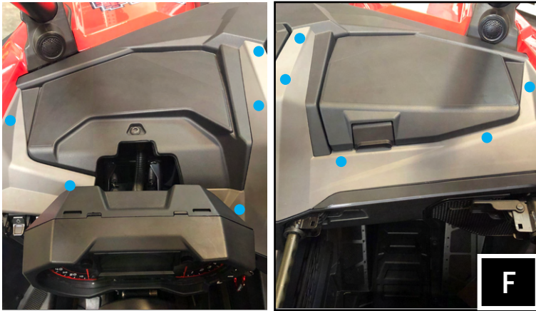
F. Use a panel tool to assist with the removal of the (3) trim panels. The blue highlighted points represent the location of the panel clips that are retaining the trim panels to the dash.
