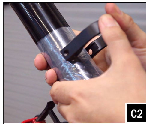
C2. Press the clamps onto the roll cage over the plastic bag.
