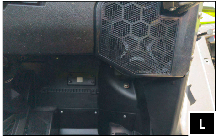
L. Reinstall the factory driver and passenger side speaker grill using the factory screws. Reinstall the front fenders.
