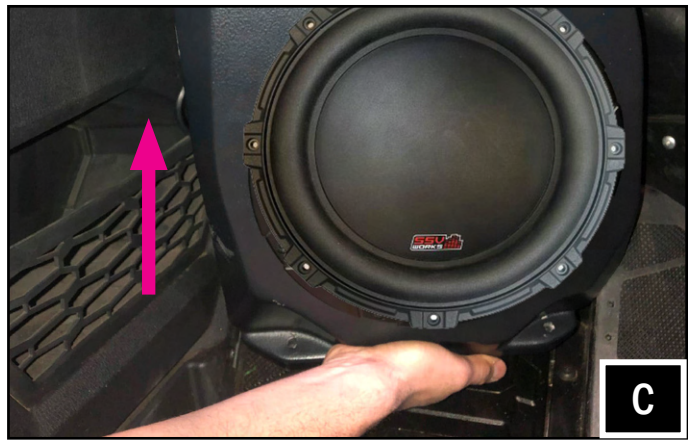
C. From the Passenger footwell, lift the 230-RZ5-UD10V into the dash cavity.
