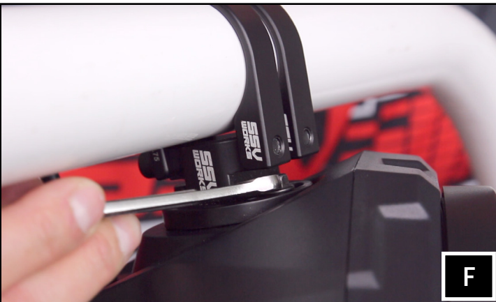
F. Position the speaker to your liking and tighten the hex head bolts by hand with a 8mm wrench.
