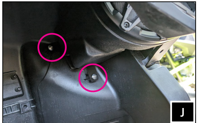
J. Secure the T brackets of each pod to the factory bosses on the footwell using (2 each) #14x.75 phillips screws [B-HP#14-4].
