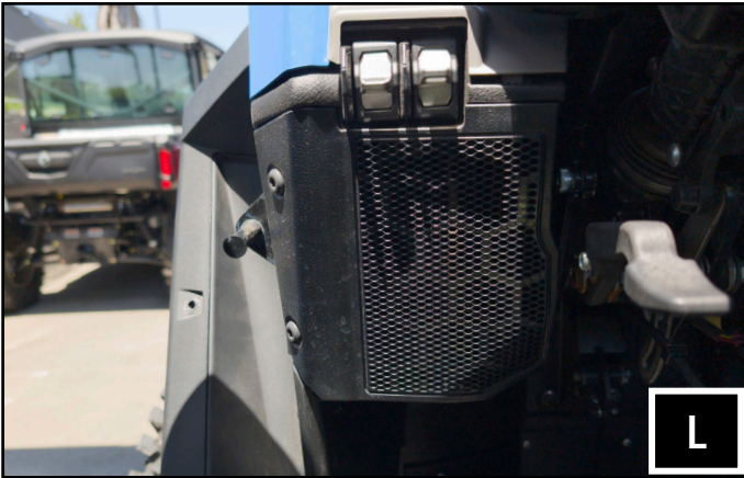
L. Reinstall the factory driver and passenger side speaker grill using the factory screws. Reinstall the front fenders.
