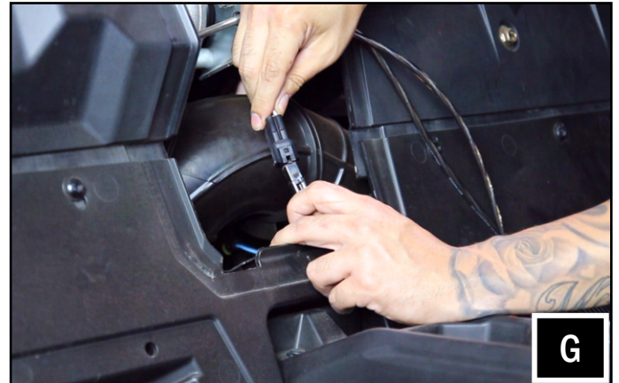
G. Take the B-H2195 rear speaker harness and plug into the B-H1913 (add B-H1912 for 4 door models) rear extension harness. Plug the B-H2936 RGB "Y" harness to B-H2933 (add B-H2934 for 4 door models) RGB extension harness.
