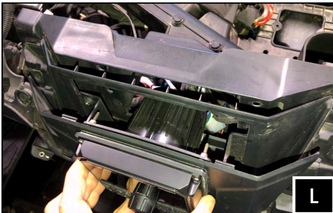
L. Place the assembled RZ5-DMR3 into the dash cavity. It is necessary to angle in one side at a time so that the bracket clears the cavity allowing the dash kit to rest flush. Now complete this step by fully tightening the screws left loose in Step D.
