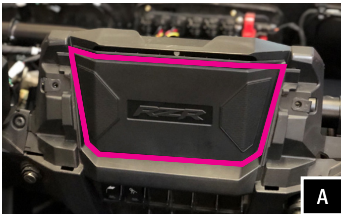
A. Use a panel tool to assist in removing the center dash cover panel
