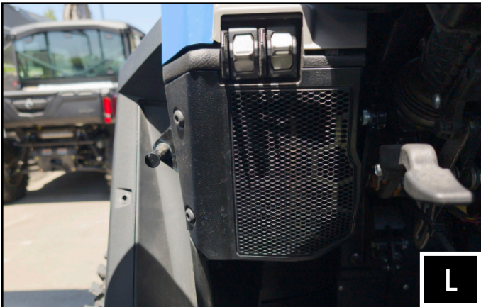
L. Reinstall the factory driver and passenger side speaker grill using the factory screws. Reinstall the front fender and any other panels that was removed.
