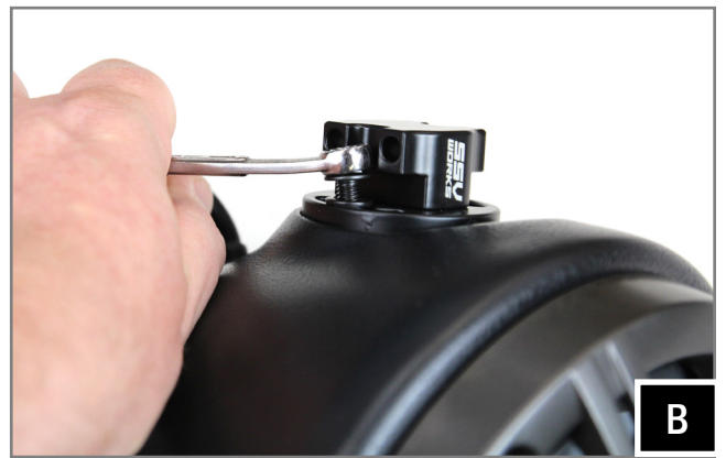
B. Loosely install the clamp base to the cage mount pod with the two (2) M6 hex head bolts and washers, place the cage mount pod in the desired mounting location on the vehicle. Once the ring adapter is in the desired position, tighten the two (2) bolts using a 8mm open wrench.
