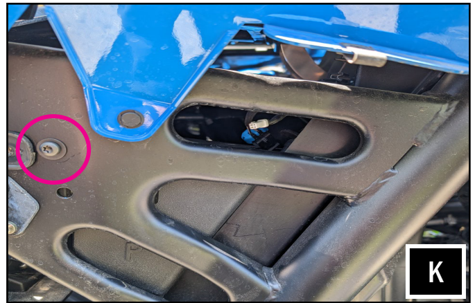
K. Secure the D (driver) and P (passenger) pod brackets to the vehicle frame using (2) M6x16 screws [B-HP3503] circled above.
