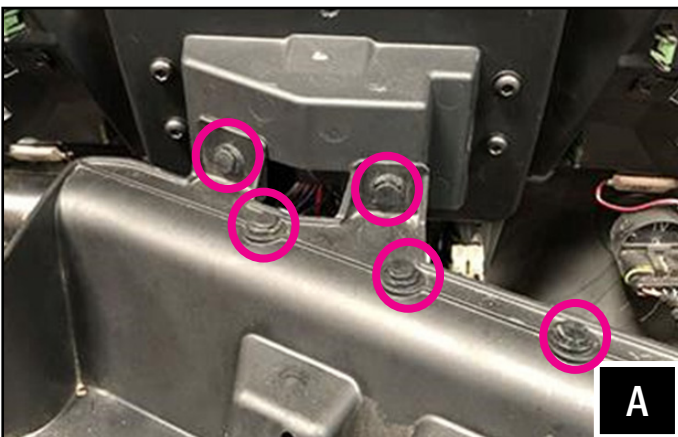
A. Remove the (5) push pins located on the plastic tray in the dash cavity.
