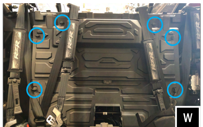
W. Twist the lock knobs on the rear firewall and remove the firewall.
