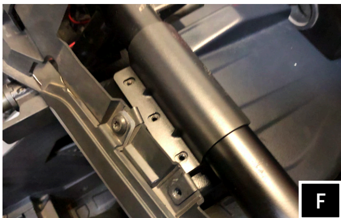
F. Place the clamp bracket over the chassis and base mounting bracket. Secure the clamp bracket to the base bracket with (3) M6x1.0x12mm T30 screws and washers.
