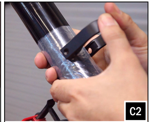
C2. Press the clamps onto the roll cage over the plastic bag.
