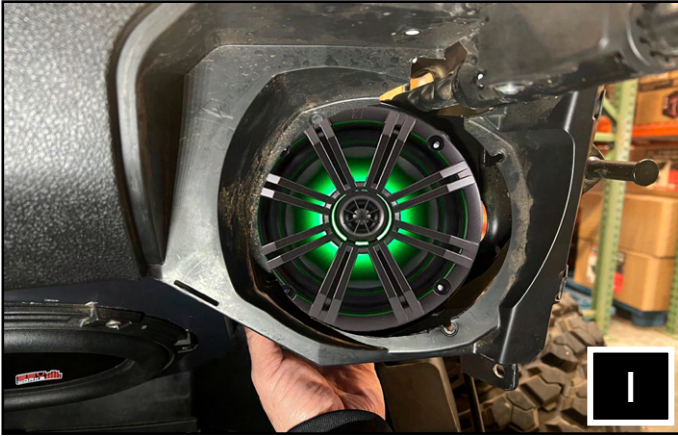
I. Slide up the RZR kick pod under the dash.
