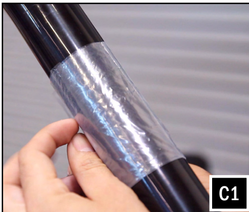
C1. Place both ring mounting clamps on the cage using the plastic bag to prevent scratching.
