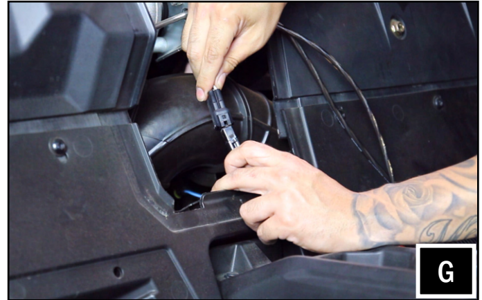
G. Take the B-H2195 rear speaker harness and plug into the B-H1913 (add B-H1912 for 4 door models) rear extension harness. Plug the B-H2936 RGB "Y" harness to B-H2933 (add B-H2934 for 4 door models) RGB extension harness.
