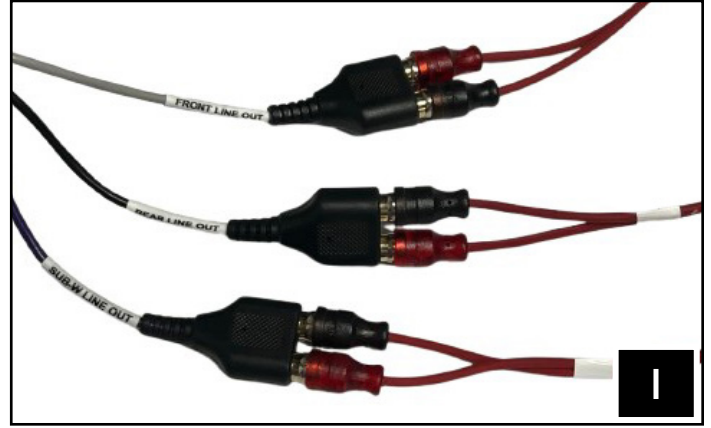
I. Plug in the B-HRCA3 to the JVC FRONT, REAR and SUB L/R Line Out RCAs.
