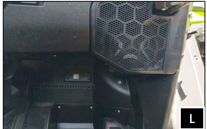
L. Reinstall the factory driver and passenger side speaker grill using the factory screws. Reinstall the front fender and any other panels that was removed.
