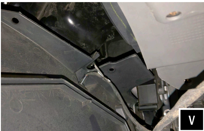
V. With the center console separated, unclip the LED from the driver and passenger console side panel. Once the LEDs have been unclipped, remove the driver console side panel from the vehicle.
