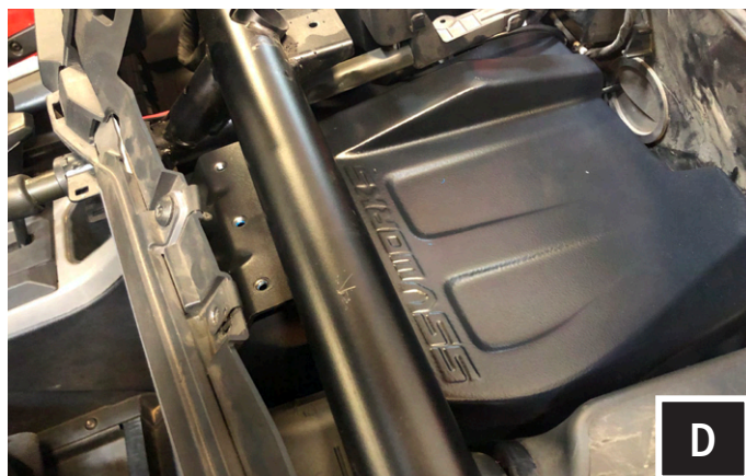
D. The top of the enclosure will tuck under the chassis cross bar. The bottom of the enclosure will rest above this edge of the firewall.
