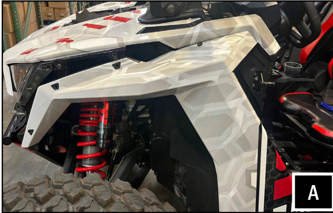
A. Start by removing the front fenders.
