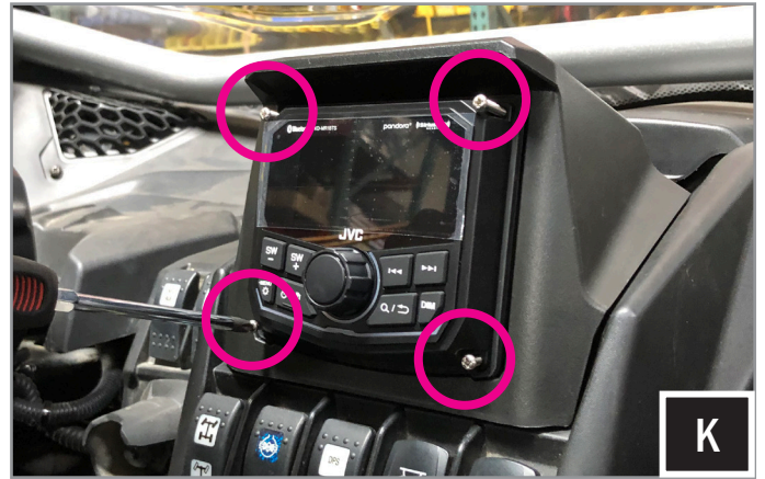
K. Secure the MR1 with the (4) M3.5 screws provided with the MR1. The top (2) screws will thread into the DMR1. The lower (2) screws will go through the DMR1 and into the threads of the base plate.
