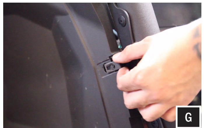
G. After the fender well panel is removed, remove the third fastener clip from the bottom.
