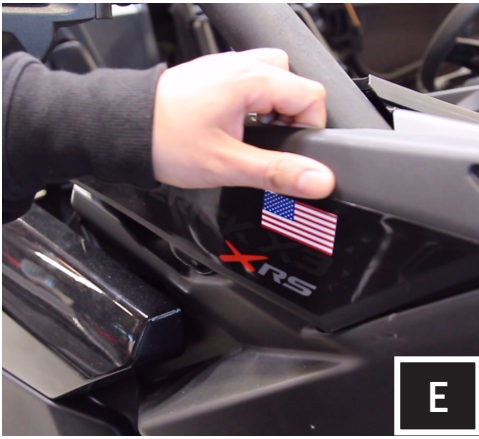
E. Remove gas cover on the passenger side to expose a 10mm nut. Unscrew with a wrench and T30 torx driver.
