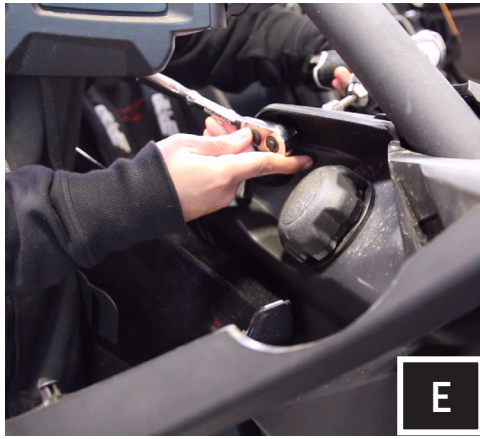
E. Remove gas cover on the passenger side to expose a 10mm nut. Unscrew with a wrench and T30 torx driver.
