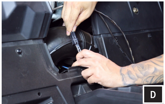
D. Take the rear speaker harness and plug into the B-H1913 & B-H1912 rear extension harness.
