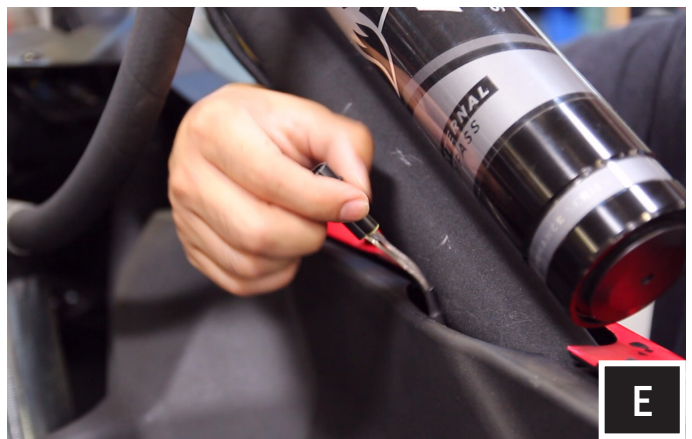
E. Route the rear "Y" speaker harness (B-H2195) along the factory wires in the engine compartment and pull up through the small space between the bed panel and cage tubing on both passenger and driver sides.
