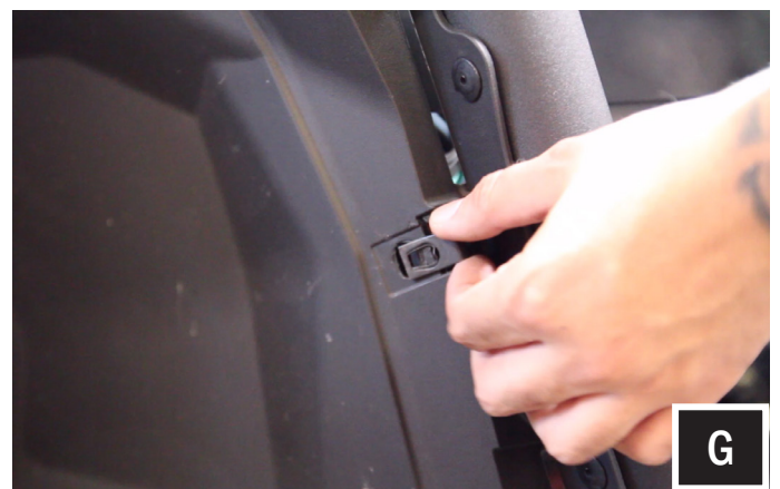
G. After the fender well panel is removed, remove the third fastener clip from the bottom.
