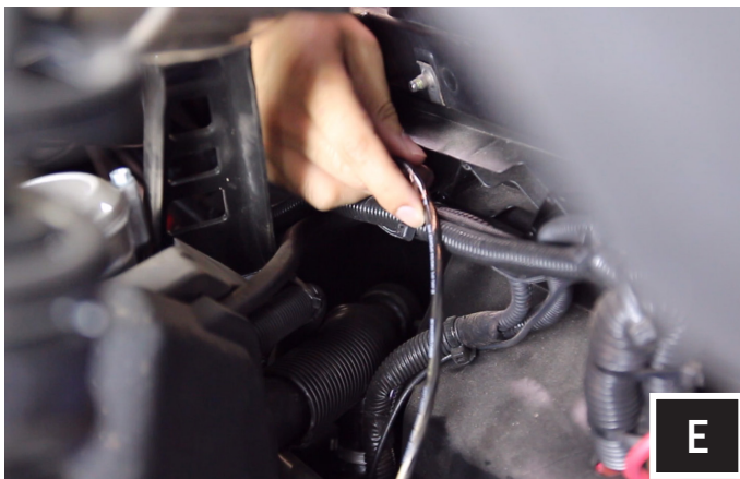
E. Route the rear "Y" speaker harness (B-H2195) along the factory wires in the engine compartment and pull up through the small space between the bed panel and cage tubing on both passenger and driver sides.
