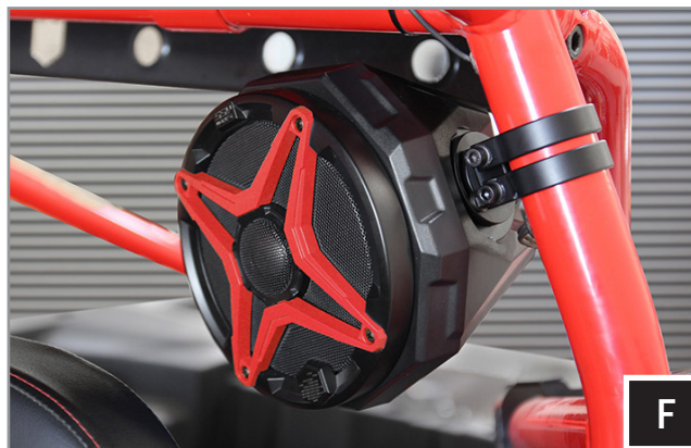
F. Route the speaker wire away from any moving parts and any sharp metal, then connect to the speaker pods.
