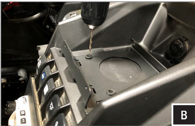
B. Using a 1/8" drill bit, drill the center of the drill guides to provide pilot holes. Limit speed and depth of the drill bit to avoid damaging any wiring.
