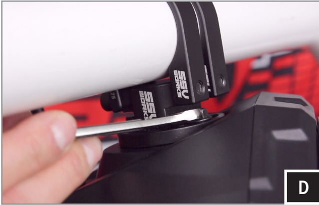
D. Position the speaker to your liking and tighten the hex head bolts by hand with a 8mm wrench.
