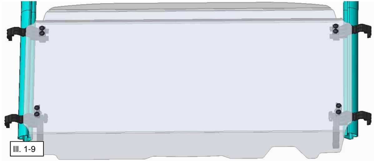
10. Loosely assemble (4) M6 x 14 Socket Heads (Item 6) connecting the clamps around the ROPS. See Illustration 1-9 & 1-10.
