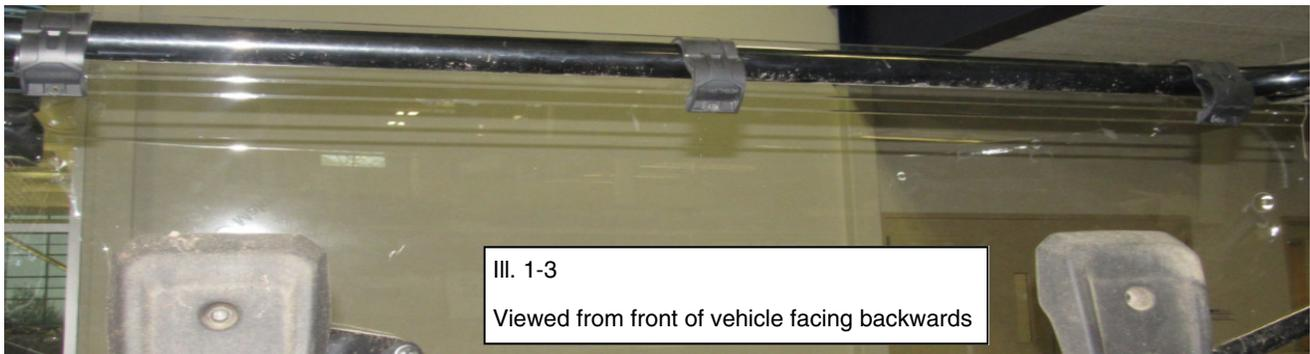
6. Insert (2) Clamp Inserts (Item 2) in each Clamp (Item 3) between the clamp and the ROPS. Install (1) M6 X 18mm Button Head Screw (Item 4) and (1) M6 Lock Washer (Item 5) into a clamp assembly to secure the clamp around the ROPS. See Illustration 1-4.
