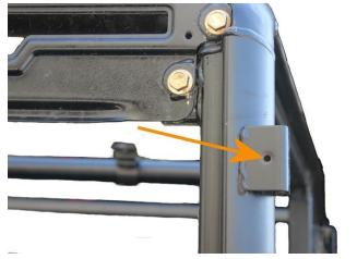
• Locate the holes to be used to install the Rear Dust Panel on the rear section of the ROPS.
