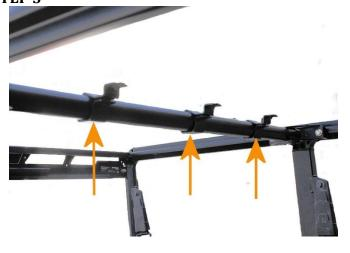
• Loosely set in place the 3 Center Roof Clamps.
