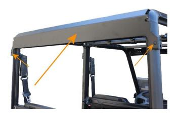
• Using the provided bolts, install the Rear Dust Panel.
