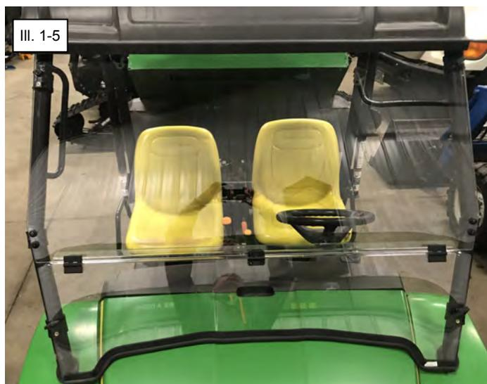
11. Check to make sure the Lower Windshield Panel can be hinged open. Adjust Windshield and re-tighten to specification if necessary. **The Lower Windshield Panel must always be in the closed position while the vehicle is moving or being transported.** The Lower Windshield should only be hinged open to access under the vehicle hood.
