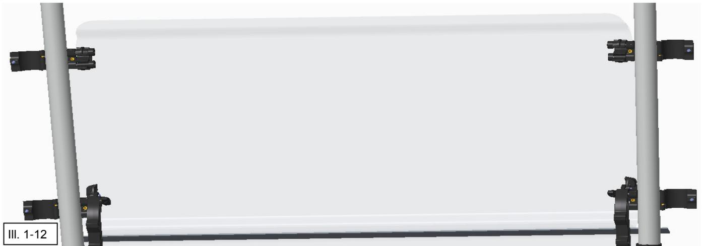
16. Loosely assemble (4) M6 x 18 Button Heads (Item 4) connecting the male & female clamp parts (Item 3) around the ROPS. See Illustration 1-13 & 1-14.
