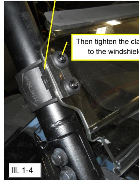
Then tighten the clamps to the windshield
