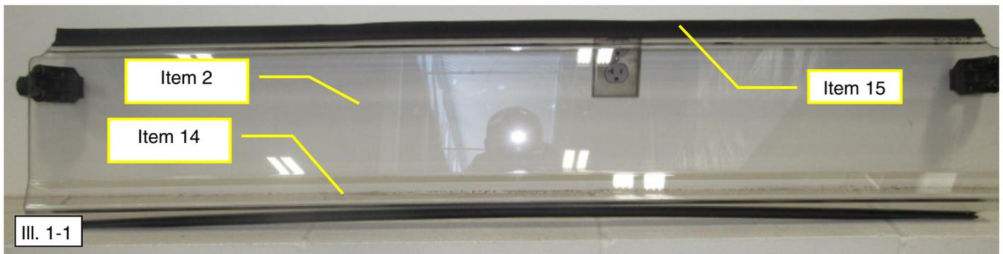
4. Assemble (1) Clamp (Item 3) on the drivers side of the Lower Windshield (Item 2) using (2) M6 x 18mm Button Heads (Item 4), (2) M6 Lock Washers (Item 5), and (2) Dome Shoulder Washers (Item 6). Do not tighten at this time to ease installation onto the vehicle. For proper fitment ensure “Kolpin” is facing outward on the clamps. Repeat for passenger’s side. See Illustration 1-2.
