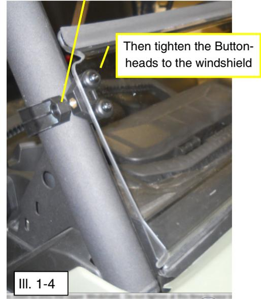
Then tighten the Button-heads to the windshield
