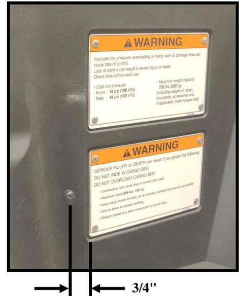
**As reference, the hole should be about 3/4" beside the lower warning label and center in height with that same warning label**
