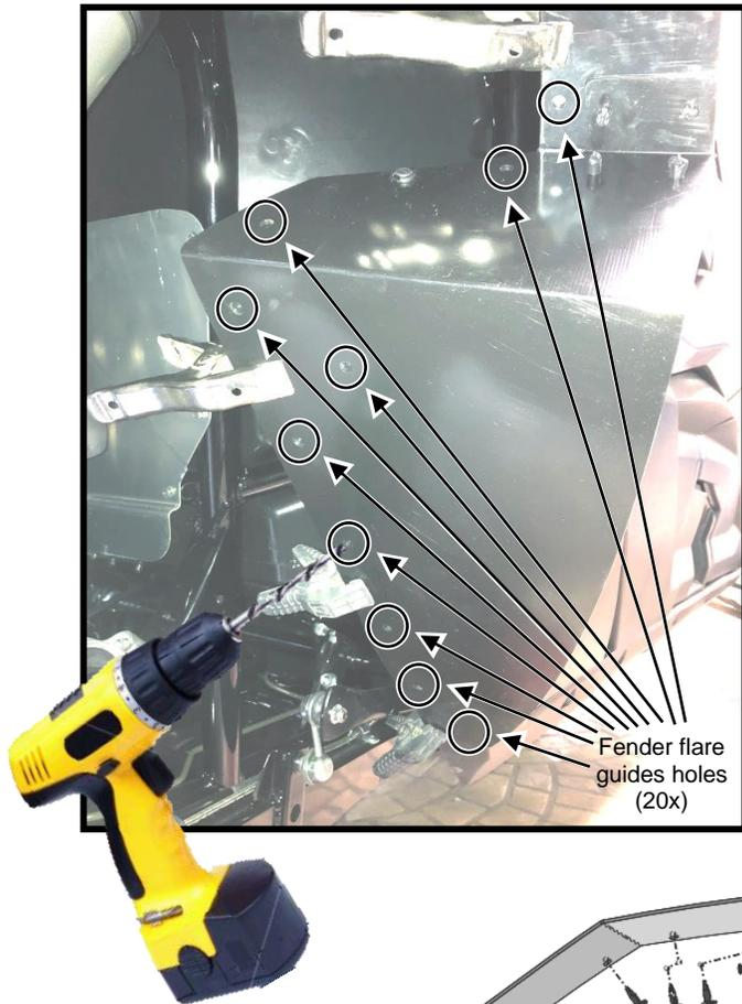
**WARNING: For each guide mounting hole, a single (1) layer of OEM rear right fender should be drilled / pierced**
