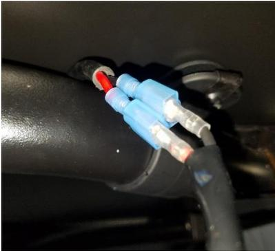
Figure 16: Harness to Light Cable Connection
