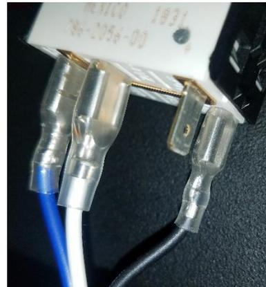
Figure 20: Proper Switch Wiring
