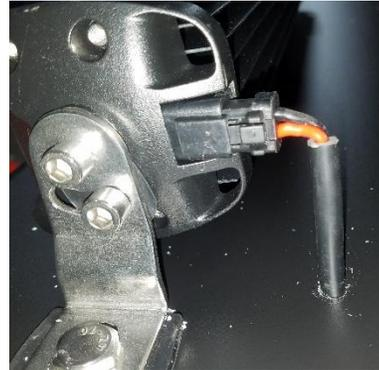
Figure 12: Routing Cable Through Roof
