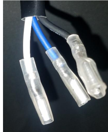
Figure 19: Switch Connectors (stock switch removed)
