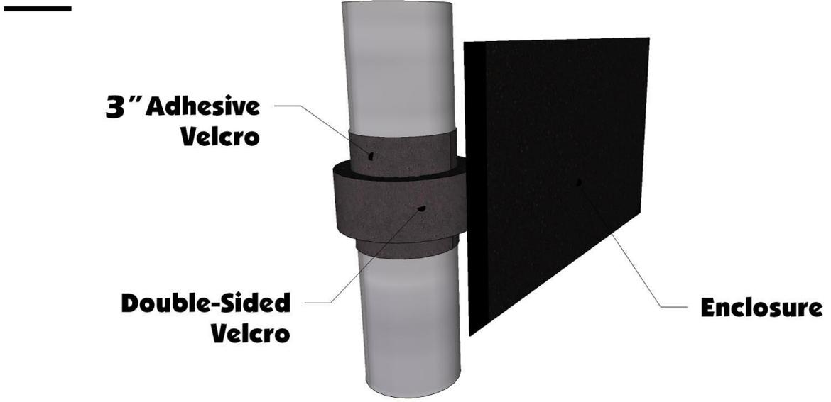
2. Once all the double-sided Velcro strips are attached all that is left is to attach the adhesive Velcro that matches up with the Velcro sewn along the bottom of the door. The rear part of the door will use the 13" adhesive strips that will go on the vehicle as shown in the picture below.
