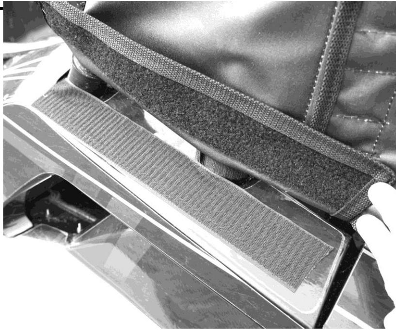
3. The bottom of the front part of the door attaches to the inside of the factory doors. Take the 27" and 13" adhesive strips and place them along the top of the doors as shown in the pictures below. NOTE: You may need to cut the strips down to make them fit correctly.
