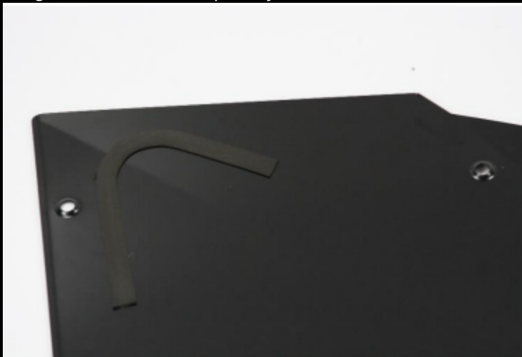
Figure 7: Foam around path of ½" tube on rear driver door
