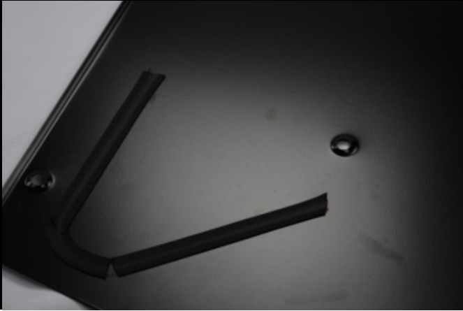
Figure 5: Foam around path of ½" tube on front driver door.
