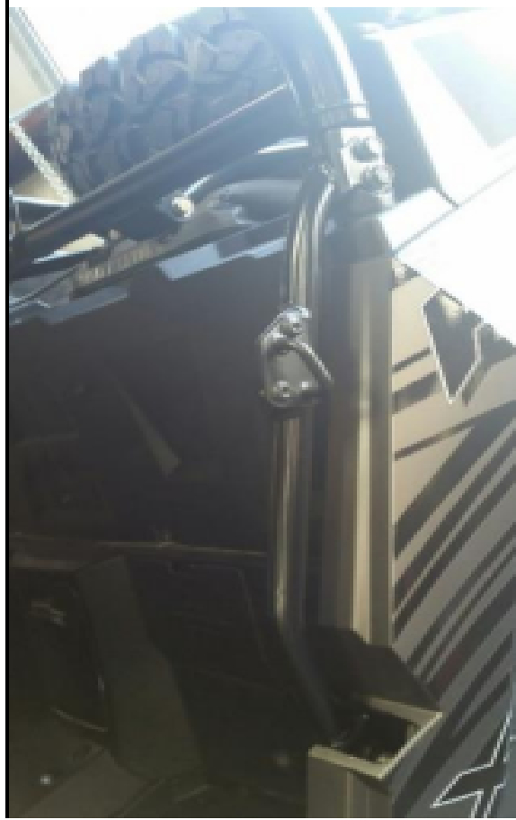
Figure 2: Rear door latch bracket mounted. Driver side shown.
