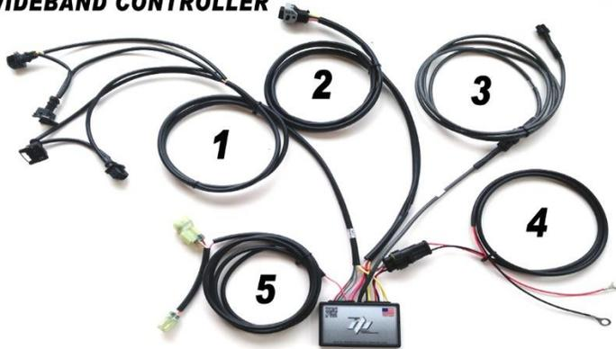
**1). Stock Fuel Injector Connector(s)** – Plugs into the factory injector connector and onto the injector to create loop around to adjust the fueling. Connector varies based on application. One male & female pair for each cylinder.
