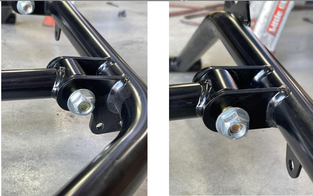
Figure 14: Fasten cross bars to swing frame tabs as shown.
