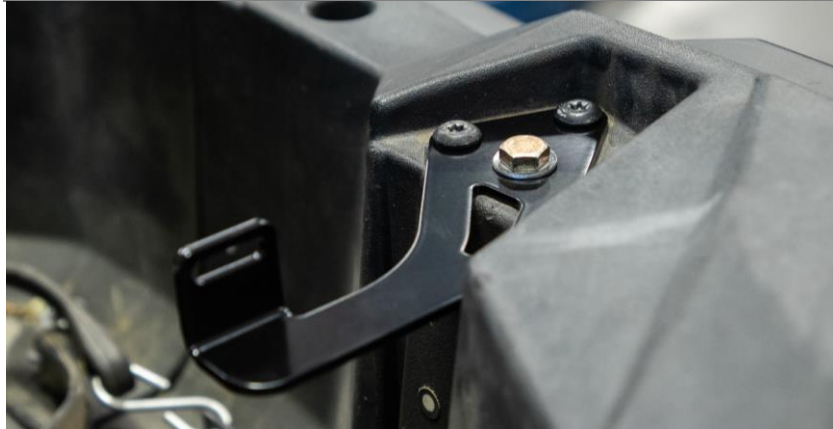
Figure 2: Flag mount brace install. Driver side shown.
