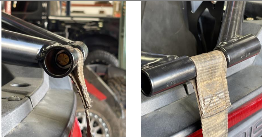
Figure 16: Connect swing frames together with supplied hardware.
