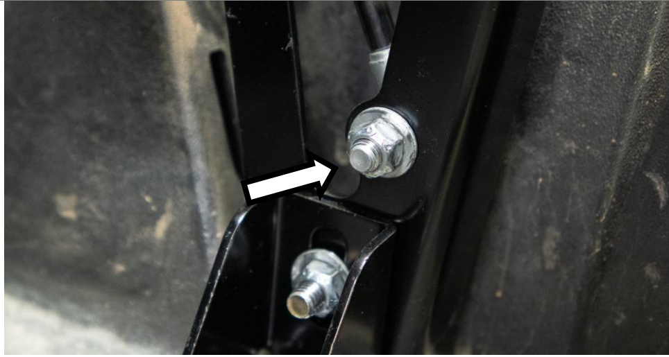
Figure 26: Insert rod end through lower support bracket. Passenger side shown.
