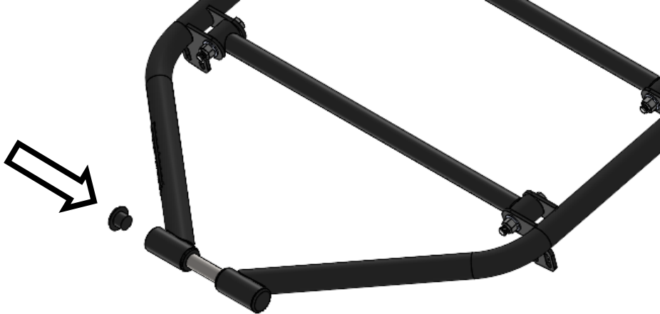
Figure 27: Plastic cap plugs pressed into swing frame.
