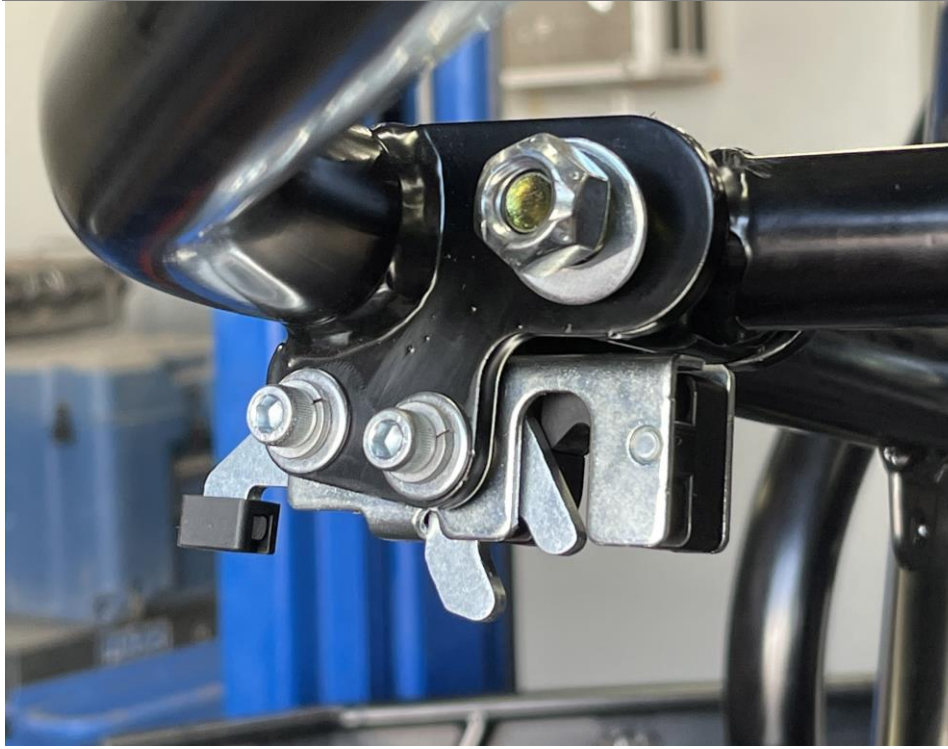
Figure 19: Latch installed onto driver side.
