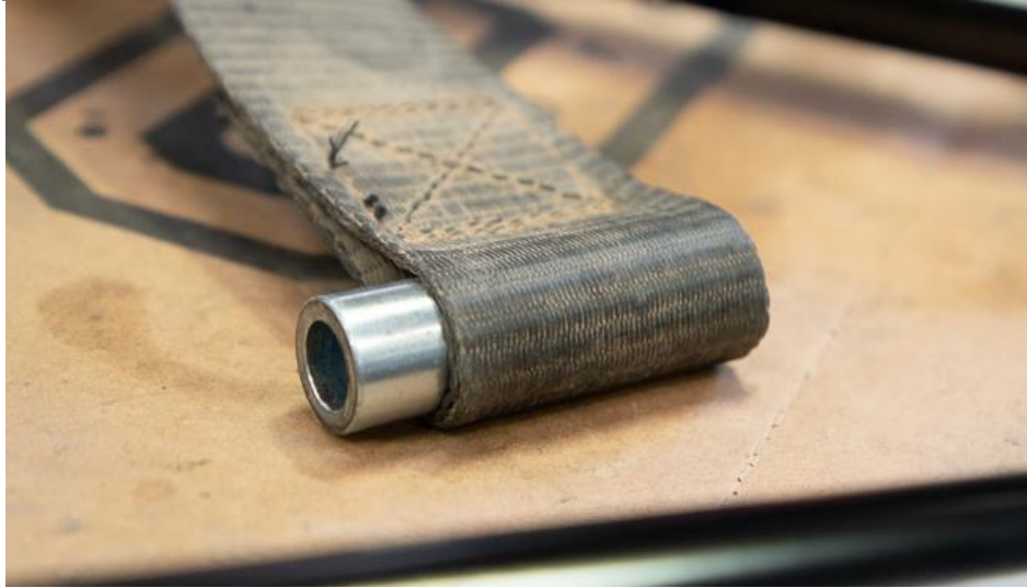
Figure 15: Insert crush sleeve into ratchet strap loop.
