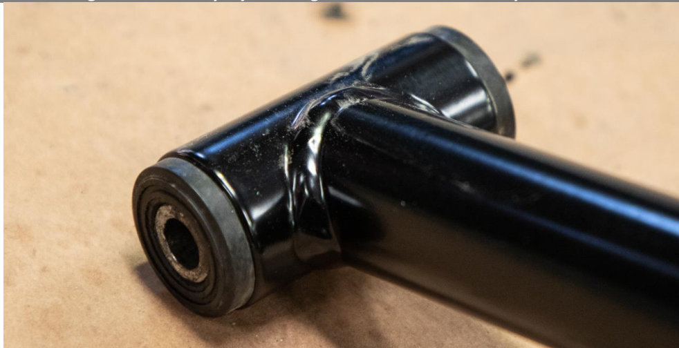
Figure 12: Insert poly bushings and crush sleeve into pivot tubes.
