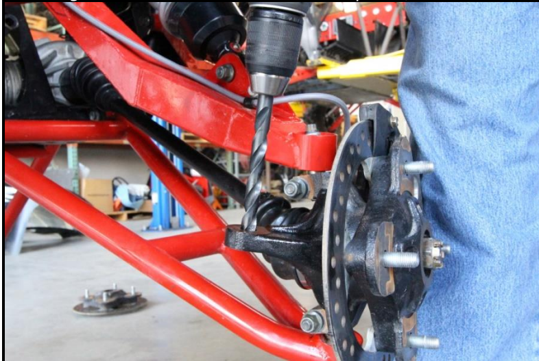
Figure 5: Drill the tie rod hole in the spindle, out to \frac{1}{2} "
