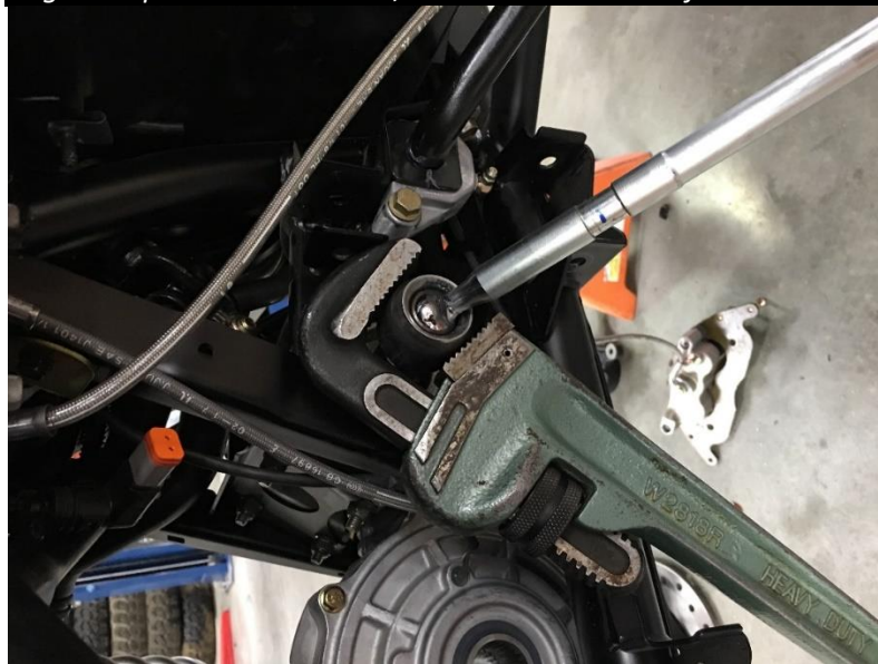
Figure 1: pull dust boot back, remove inner tie rod from rack bar.
