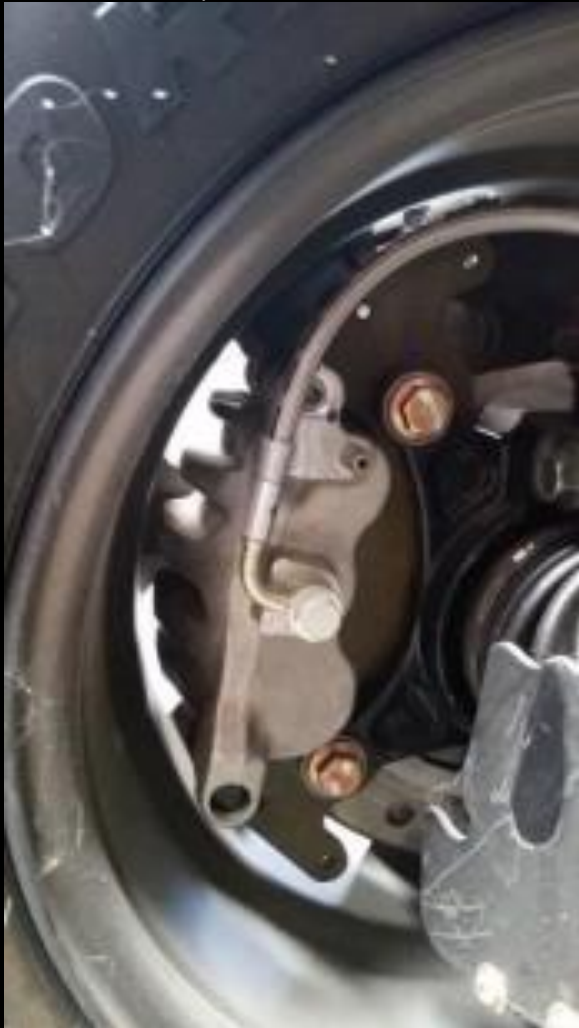
Figure 5: This is stock. The brake line fitting is far from the bleeder screw, this kicks the brake line up close to the wheel.
