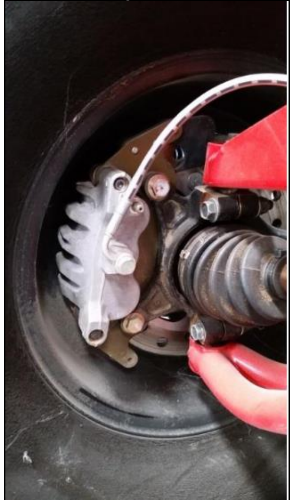
Figure 6: loosen the bolt a tad, just enough to turn the fitting closer to the bleeder as shown, retighten bolt.
