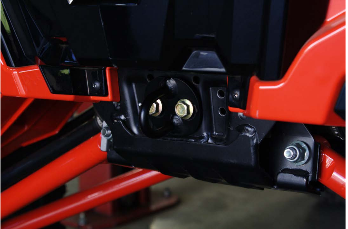
Figure 1: The OEM Tow Loop is held by two 10mm bolts.
