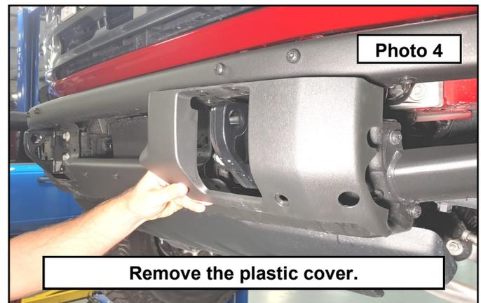
8. If you have proximity sensors in your bumper, disconnect their harness. Behind the plastic cover you will find the main bumper mounting hardware. Have an assistant help hold the bumper and remove the 6 mounting bolts using a 15mm socket. **Photo 5**
