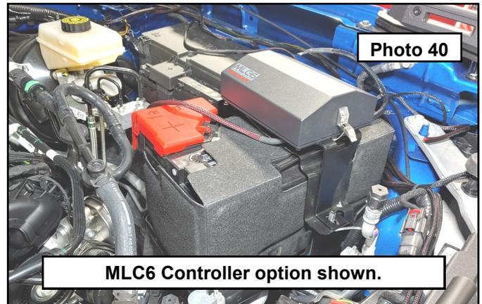
37. If you do not use the MLC6 unit, you can attach the light bar and cube harnesses to the aux switch wires under the hood. You will need to cut the switch end of the harness and use the trigger wire to attach to the AUX wires coming from the vehicle. In this you will find a blue, black and white wire. Pull the protective sleeve cover from the relay to access the wires. Find the color wire that is doubled up with the Red power wire going to the relay. **Photo 41**
