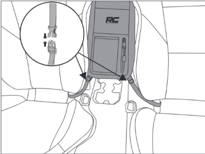
3. Wrap two bottom straps on seat frame and fasten the buckles.
