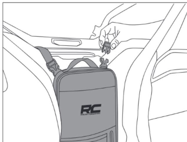
2. Wrap two top straps on frame bar behind the seats. Then fasten the buckles.
