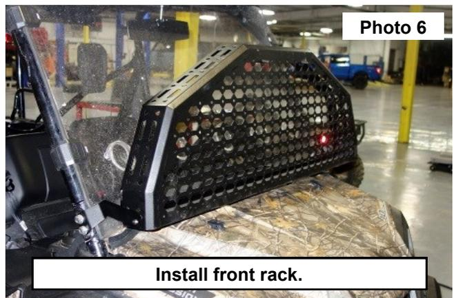
5. Place the front support bracket on the bumper bar and lower the front rack down and install the supplied 8mm bolts, nuts, and washers. **See Photo 7 and Photo 8.**
