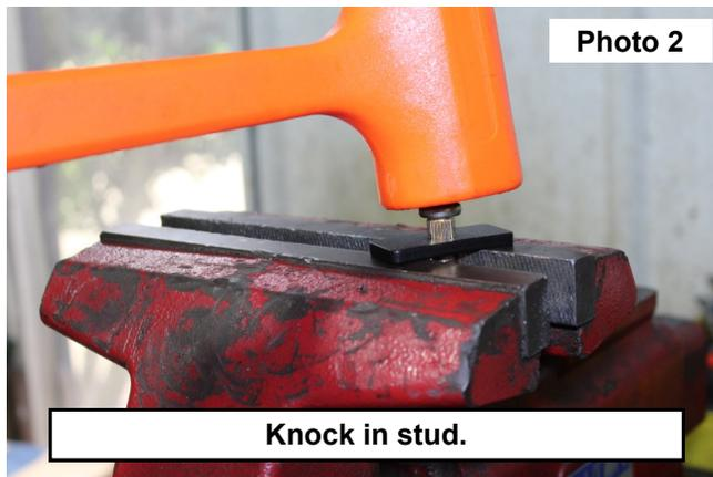
3. Make sure bottom flange of 10mm stud is flush to bolt plate. **See Photo 3.**
