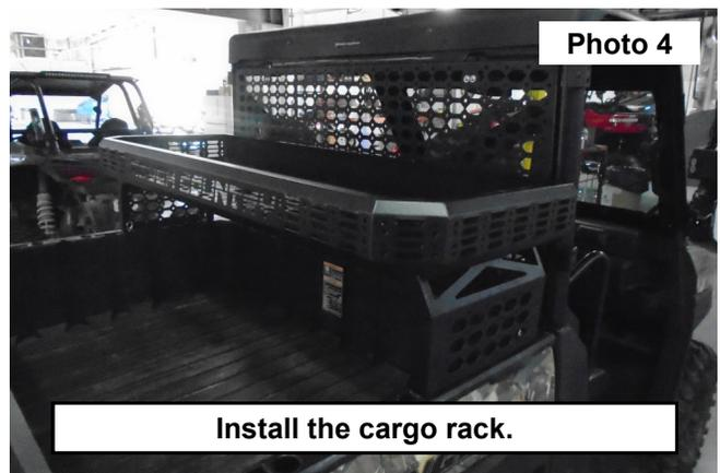
5. Using the Supplied hardware secure the cargo rack to the side panels. Tighten using a 13mm socket and a 5mm Allen wrench. **See Photos 5 and 6.**
