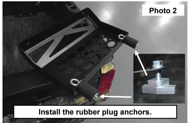
3. Place the rubber plug anchor or T Mounts on side panels into the bed on each side of the UTV. **See Photo 3.**
