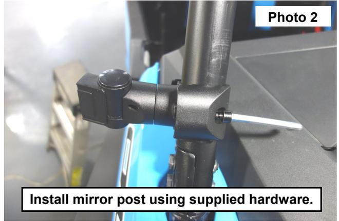
3. Insert the mirror into the mirror post and secure using the supplied bolts and Allen wrench. **See Photo 3 and Photo 4.**
