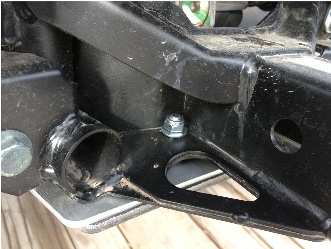
Step thirteen: Now you can mount your top plate. (775T) The front mounting points on the frame are not threaded from the factory. We supply a M6 self tapping bolt for these
