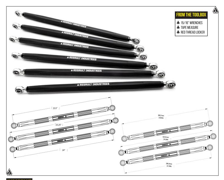
Prior to removal of OEM radius rods, take measurements from the center-point of the bolt hole from end to end on each rod. Note the measurements as each radius rod should be preset to the appropriate length prior to installation to save time.
