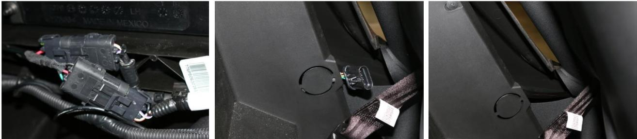
4. **Run the other end** - of the rear harness to the front kick panel. The plastic has a perforated circle behind the driver's seat or rear seat behind the driver on the MAX, at this location you can push the rear harness single connector through the plastic gap to the passenger compartment, follow the frame along the driver's side, the harness can be hidden in the side panels and goes up behind the removed kick panel and plug it into the mating connector on the Control Module.
