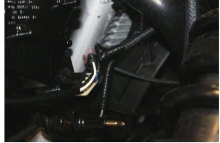
7. **Attach Front Harness to lights** - The Green and white wire go to the right/passenger side LED, attach the Green to the Black and the White to the White, the Yellow and white wire go to the Left/Driver side LED, attach the yellow to the Black and the white to the White (above right photo). NOTE: Black wire is positive and go to the Green and Yellow, they will not work if reversed. White is ground. Secure the Harness using the provided cable ties.
