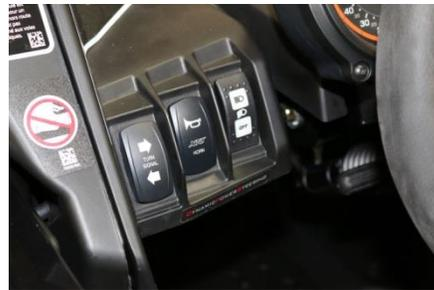
9. **Install Hazard/Horn Switch** - - Remove one of the switch blanks and run our 10-pin switch connector through the opening, grease the terminals with the supplied grease and attach to Hazard/Horn switch and insert the switch into the opening.
