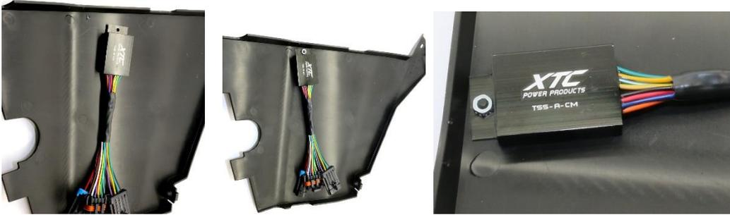
3. **Run the Rear Harness** - Starting at the rear driver’s side light harness, these connections are on the plastic wall in the front engine area, take the end of the cable with two connectors on it and run it from the OEM Rear Light Harness on the Driver's side to the OEM Rear Light Harness on the Passenger side, follow the factory wiring, unplug both harness and install our harness into the factory harness. Secure using the supplied cable ties
