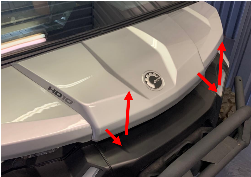
Figure 12: Remove the radiator hood access panel.
